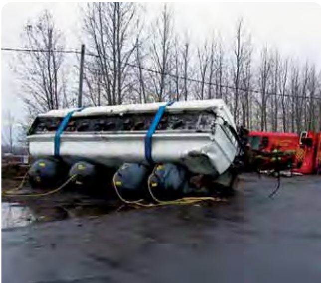
Efficient lifting of overturned vehicles.
