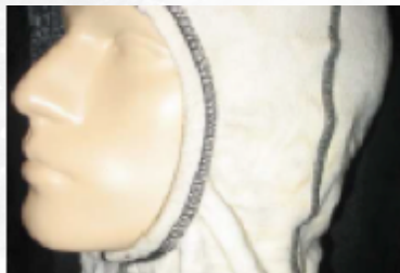
Hood inside out – this side with Nomex® Nano Flex
