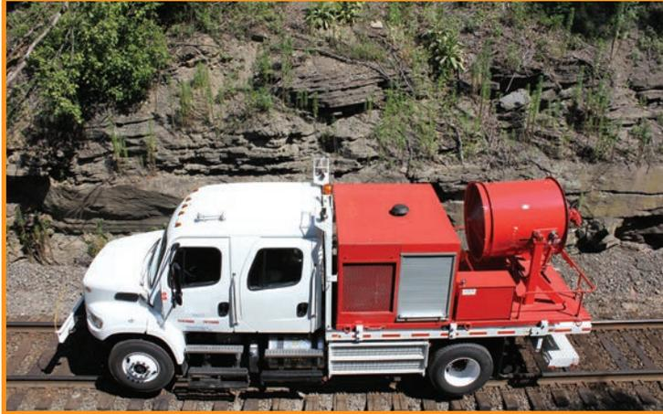
Like the MVU®-60, all of the 48's mechanical actions, including the fan's blade rotation, are powered by a reliable hydraulic system. The hydraulic pressures are generated by its turbo charged engine, mounted under the MVU®'s silencer hood. Every MVU®-48 is custom built by our team of engineers and fabricators.
