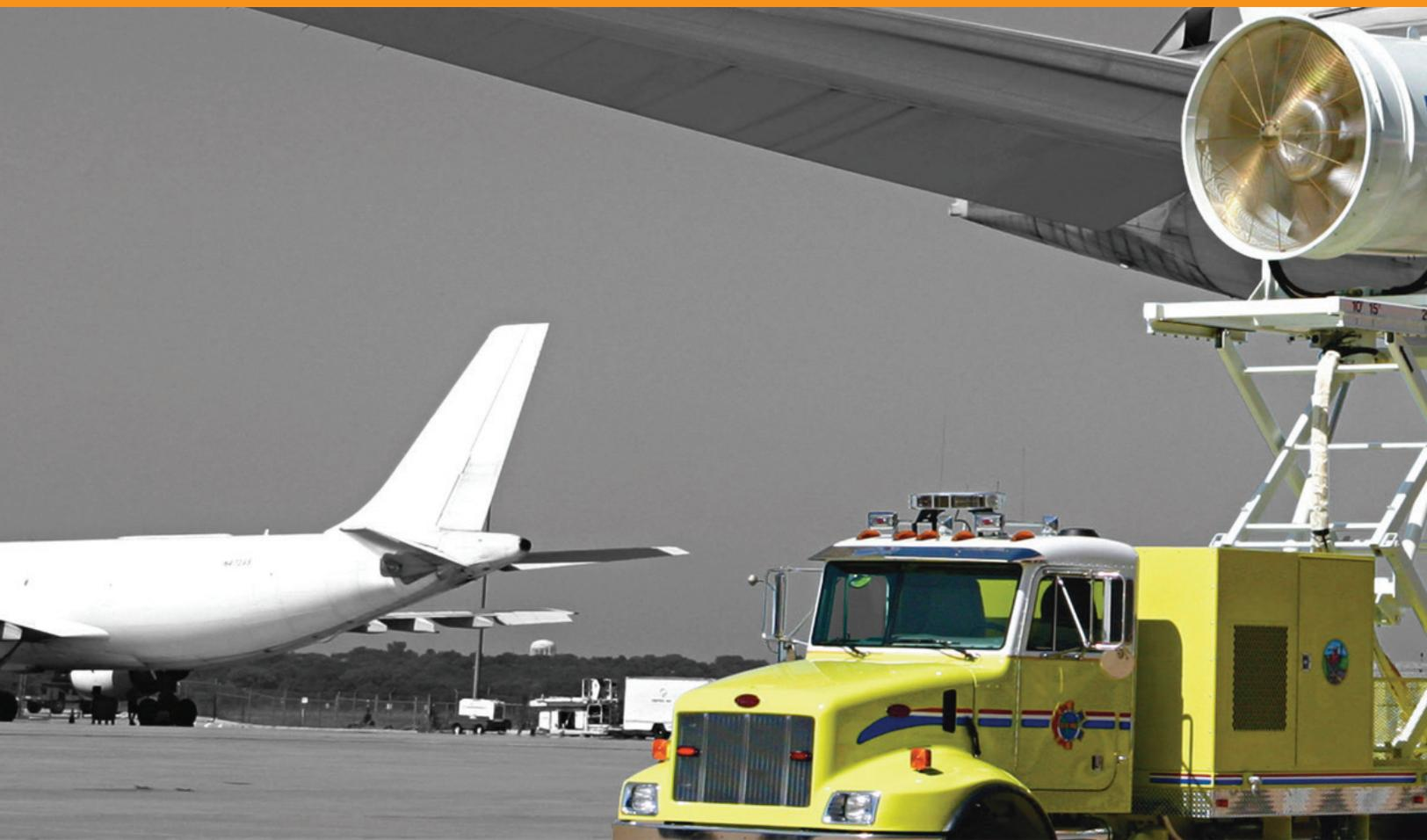
The powerhouse of our ventilation line, the **TEMPEST MVU® 60** is the largest unit we manufacture. The combined massive 60" (1.5 meters) seven (7) blade aluminum impeller, and steel shroud are capable of generating air movement unlike any other ventilation unit. At a calculated 400,000 Open Air Flow CFM (679,000 m<sup>3</sup>/hr), the MVU®60 will ventilate nearly anything caught downwind from it.
