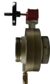
Gear operator handwheel must be mounted on the right or left side of the valve body for the valve disk open-closed indicator to show the correct position of the valve disk. If the gearbox is mounted so the handwheel is in front of the valve, the open-closed indicator will not indicate the correct position of the valve disk. An optional valve shaft is available to correct this problem. Please call our customer service department for more information.
